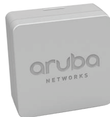
Figure 3: IP67 Rated Outdoor Case
