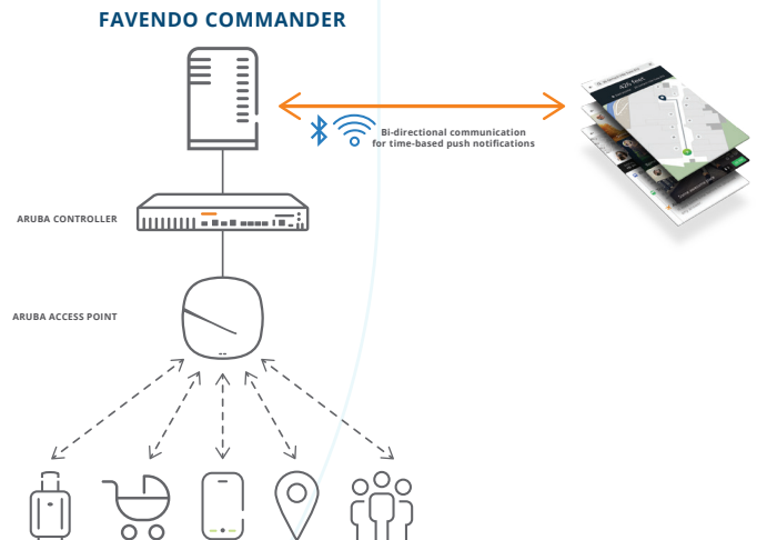
Figure 31: Aruba and Favendo joint solution topology
