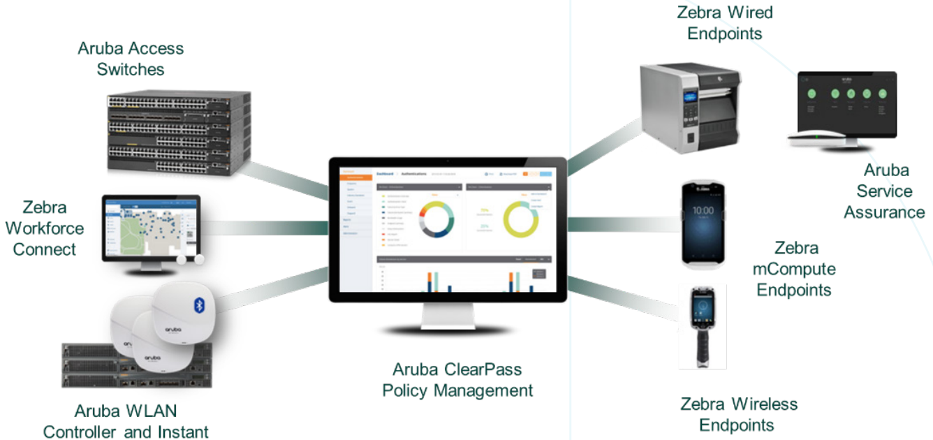
Figure 28: Aruba-Zebra Integrated Voice and Data Capture
